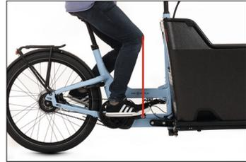
Sit on the CD2 in the position shown above with horizontal crank arms and have a second person determine the knee plumb line.
