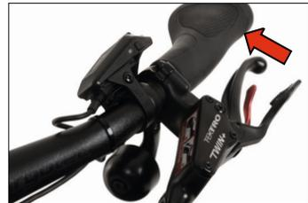
The brake system has fully automatic pad compensation. This compensates for the wear of the brake pads and ensures that the pressure point of the brake always remains the same.
