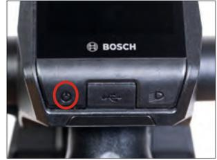
To switch off, press the power button for at least 3 seconds.
