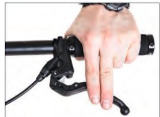
By loosening the screw on the handlebar clamp, the brake lever can be moved on the handlebar. When you have found the right position, first tighten the grips only enough so that they can still be turned. In the next step, adjust the angle of the brake handles. You may also first have to loosen and move the Bosch control unit with a suitable Allen key.
