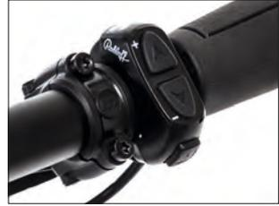
If the pedelec is stopped from a speed of more than 10 km/h, the system can automatically shift back to a set "start gear". To set the starting gear, please refer to the corresponding enclosed Bosch instructions.
