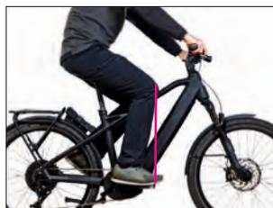
Sit on the vehicle in the position shown above with horizontal crank arms and let a second person determine the knee plumb line
