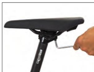
Set the tilt of the saddle horizontally or with the saddle tip inclined downwards slightly. Then tighten the screws with 10-12 Nm.
