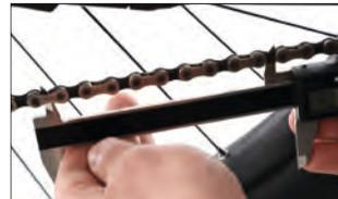
With a length more than 120.5 mm, the chain is worn to such an extent that the chainring and sprocket wear excessively. In this case replace the chain with a new one.
