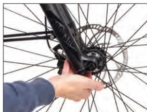
Turn the quick-release lever to tighten the axle. Fold the quick-release lever over at the end.
